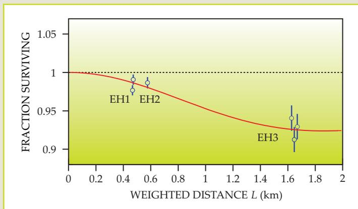
**Figure 2. Observed fraction** of the  $\bar{\nu}_e$  flux expected at each detector in the absence of neutrino oscillation is plotted against the effective mean distance of each experimental hall (EH) from the six reactors that produce the antineutrinos. The curve shows the prediction from the best neutrino-oscillation fit to the flux-shortfall data. (Adapted from ref. 1.)
