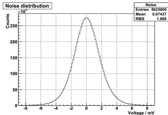
Figure 3: Electronics noise of a typical readout channel after DRS calibration
