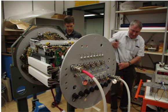
Figure 1: Ongoing final assembly of the FACT camera at ETH Zurich. The compact compartment houses the complete trigger and readout electronics for 1440 pixels
