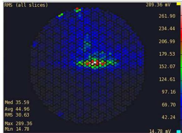
Figure 7: Triggered camera image induced by a signal from a light pulser integrated in the camera lid.
