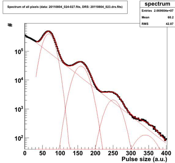
Figure 6: Combined dark count spectrum of 1435 G-APDs. Only DRS calibration was applied. The dark count spectrum is identical to a single photon spectrum
