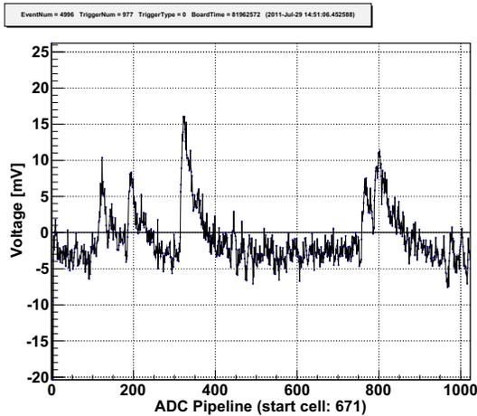
Figure 5: Readout of a single pixel with closed camera lid and random trigger. The DRS-4 was operated with 2 GHz, i.e. each channel corresponds to 0.5 ns. See text for description.
