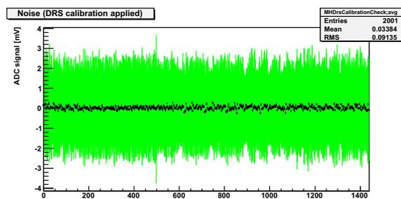
Figure 4: Electronics noise of all readout channel after DRS calibration
