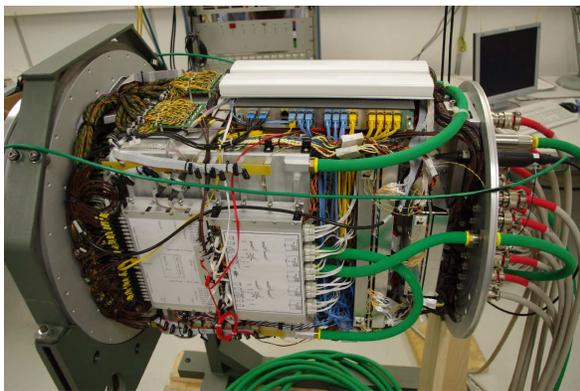
Figure 2: Completely assembled FACT camera during tests at ETH Zurich, shortly before the cover was closed. The thick cables at the backside deliver the 320 different bias voltages to individual pixel groups.
