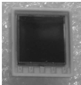
Figure 1: A 2 \times 2 monolithic array of 3 mm square MPPCs (Type=S10985-050C(X), ID=5).
