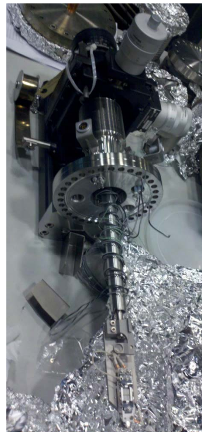
VG五维真空样品架：可原位加热或降温
